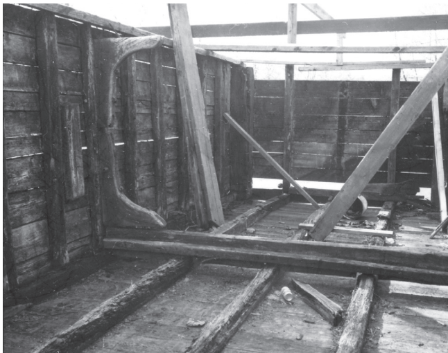
BELOW: This interior view, taken at about the same time as the photo above, shows the boat's frame and heavy planking. The light showing between her planks indicates the oakum that once sealed her seams had long since rotted away.
